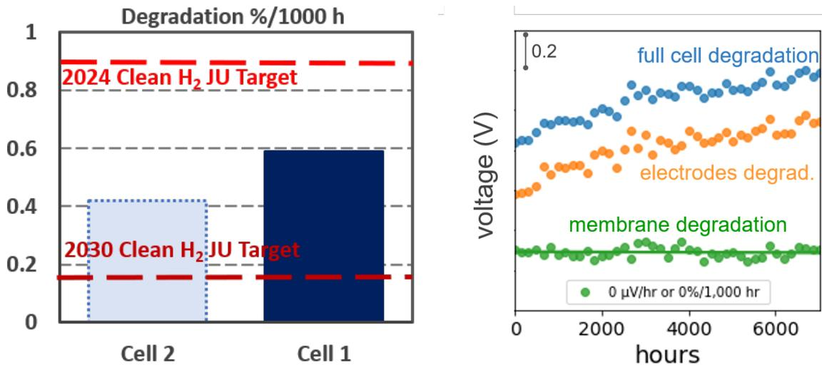
Aemion+® membranes were assembled in Ionomr's nickel-based large-format, 50 cm<sup>2</sup> active area electrolyzer test hardware equipped with leading commercial alkaline electrodes, known for their long life and stable operation for up to 20 years. This approach allows for the evaluation of the durability of the membrane independent of the catalyst layer, unlike alternative approaches such as a catalyst-coated membrane.
